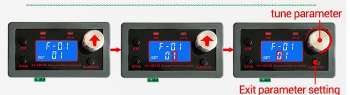
In the menu setting interface, short press the encoder to enter the F-XX corresponding menu parameter setting state, the parameter flashes, short press again to shift, rotate the encoder to adjust the parameters. Short press the RUN/STOP button to exit the parameter setting and return to the main menu number adjustment interface.
